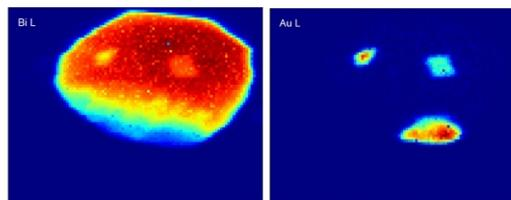
Bismuth grain (3  $\mu\text{m}$  across) with extremely fine-grained gold. The nano-XRF image pixel size is 50 nm.
