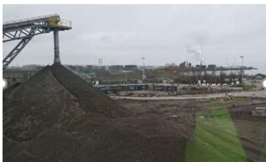
Figure. The storage of processed ash at SYSAVs facility at Spillepengen, Malmö
