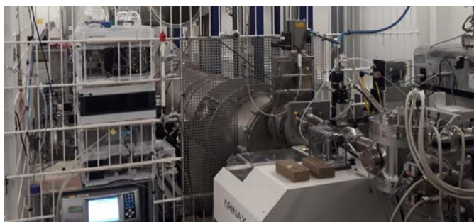
Figure 11 The beamline P12 at EMBL Hamburg allows studying the structure of molecules in solution using small-angle X-ray scattering (SAXS) technique. (Svergun group/EMBL)
