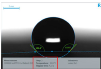
Imaging from the measurements: The drops remain spherical on the textile surface at a contact angle of 140° and hardly adhere to it (Images: research consortium)
