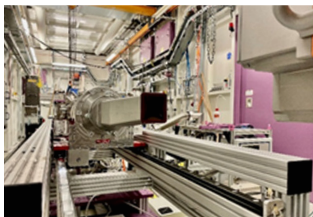
Figure 2: WAXS detector (top right) and flight tube for the USAXS detector (in the middle), at the beamline P03 at PETRA III.
